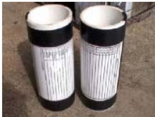
Figure 17. Slates made out of PVC pipes that are put over the lower arm of the observer. This type of slate is convenient for use in areas that are prone to strong currents.
