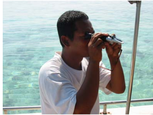
Figure 11. Purwanto uses the refractometer to measure water salinity for SeagrassNet monitoring.
